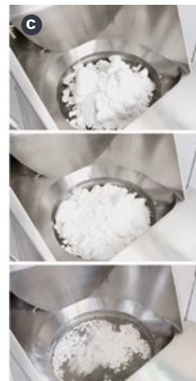
C: Sieving process in the sack discharger
